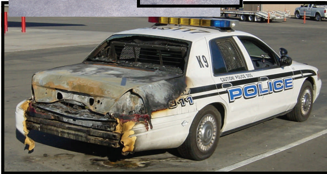
Accidental Combustion of Fusee Flares in Trunk of Police Car
